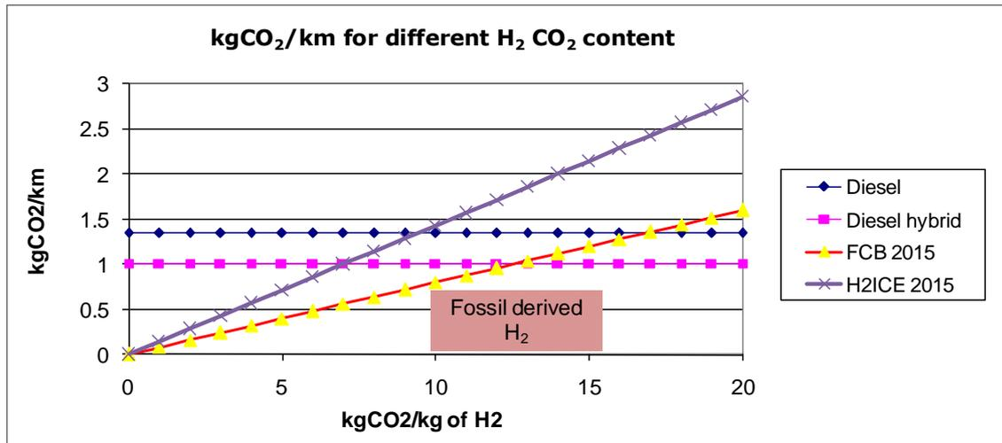
*Illustration of the well to wheel CO<sub>2</sub> emissions for a 12m single deck bus for four different drivetrains in 2015, for different CO<sub>2</sub> content hydrogen. The assumptions on fuel economy are – diesel 45l/100km, diesel hybrid 34l/100km, fuel cell hybrid 8kg/100km, H2ICE hybrid 14kg/100km.*
