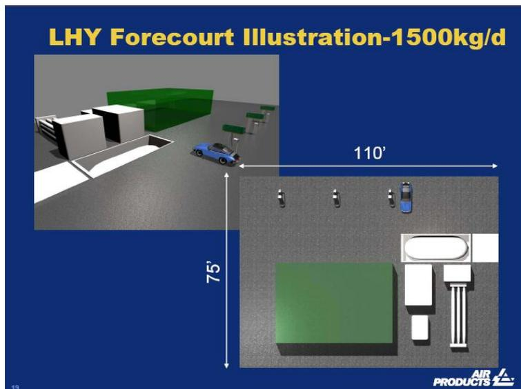
*Illustration of footprints for different hydrogen filling solutions at a demand of 1,500 kg/day.*
